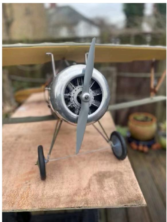
My Legionnaire had it's first proper assembly at home the other day. It's sporting an OS four stroke 40 engine swinging a 12 x 5 prop. I balanced it by moving the receiver battery around but it may be some time before the weather is kind enough for its maiden flight.
