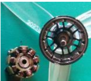
Figure 7 Disassembled motor that produced flam
