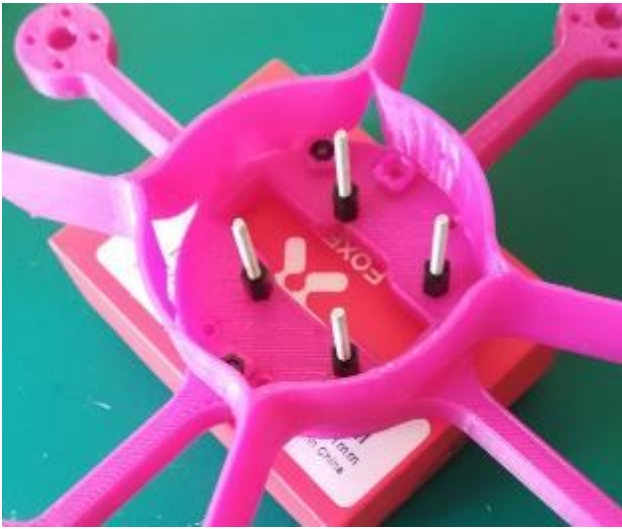
Figure 4 Remixed design main body with dry fitted components
