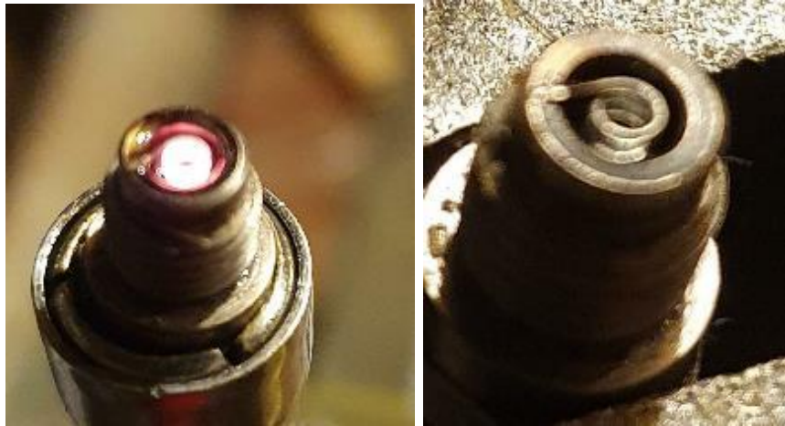
Appears to glow nicely but the element has a dull coating effecting performance
