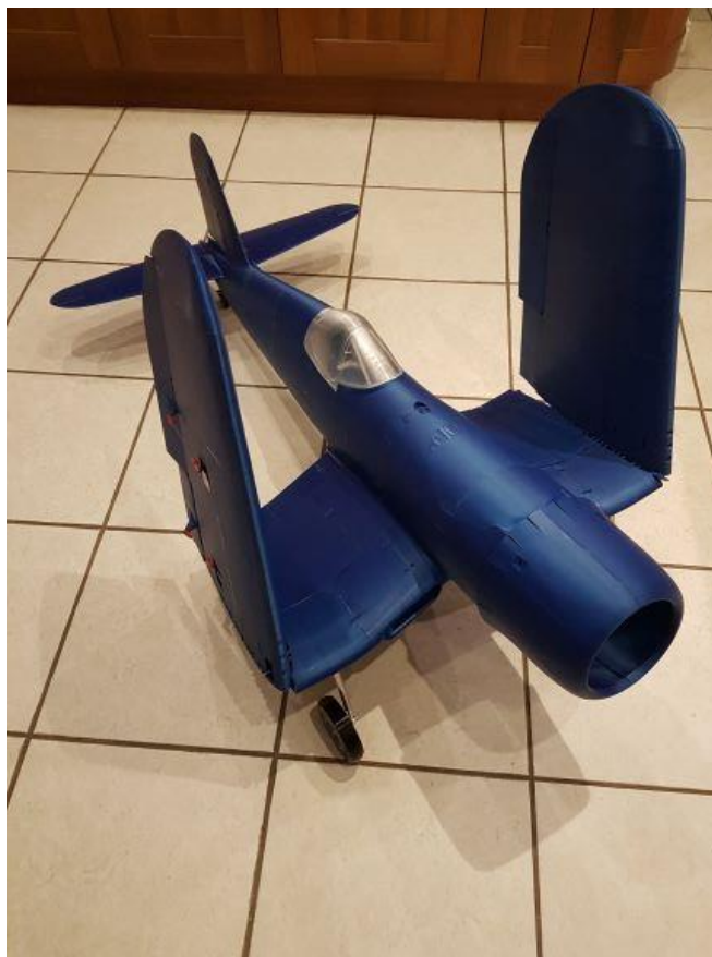
Folding wings are held on with 2 PLA pins each side.
