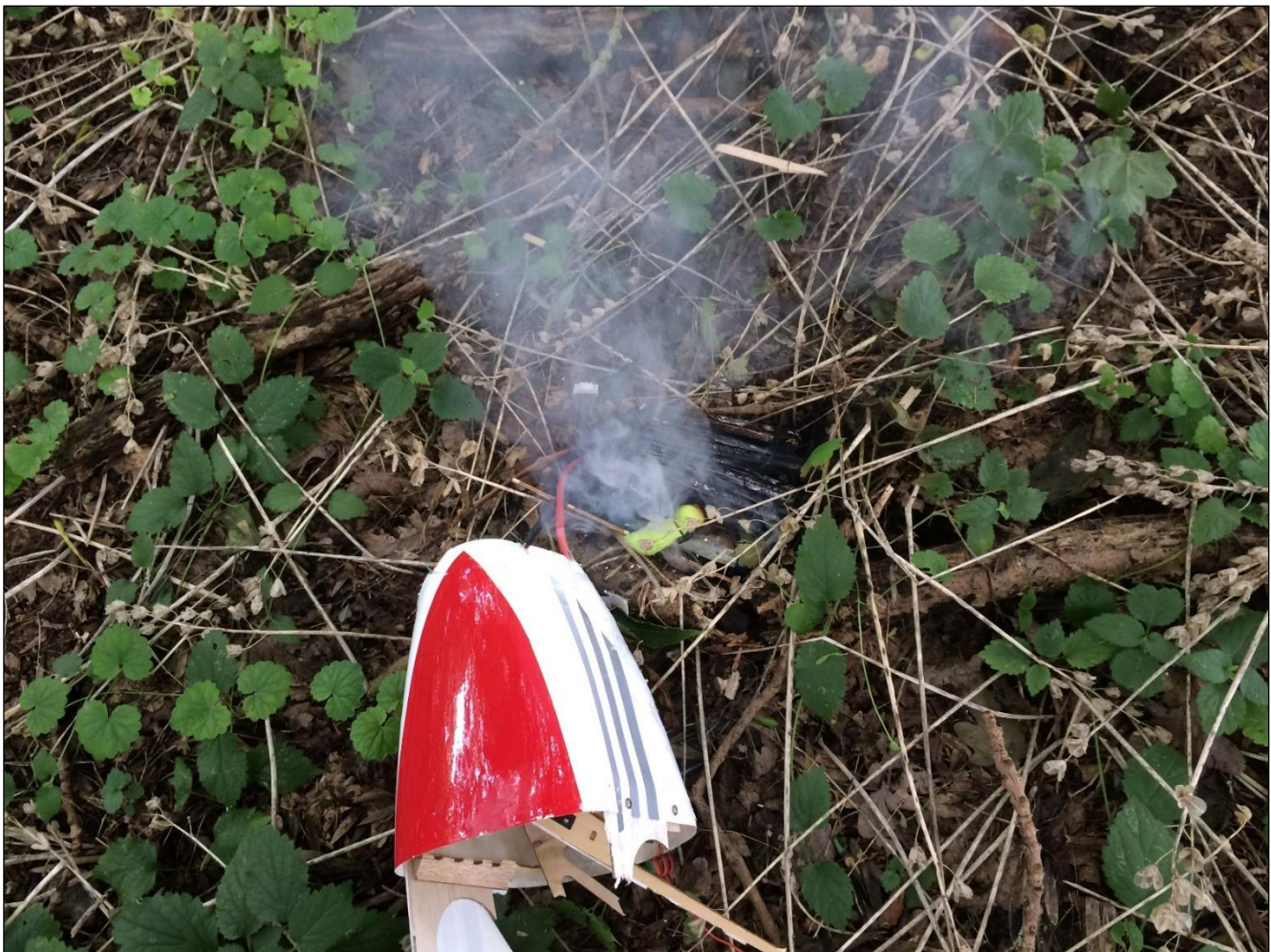
This is what a burned 6s4200 LiPo looks like; first time it's happened to me, actually, but I suppose that fire is always a risk after a crash that involves a LiPo..
