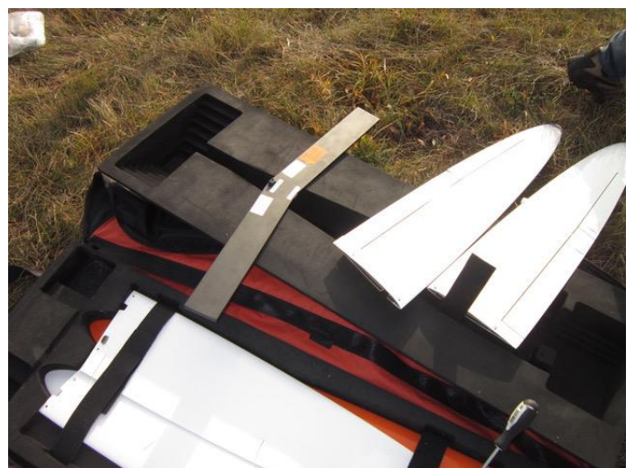
Here we have the flight battery (the boomerang shape) which fits into the wing, the connection is made when you bolt the wings onto the fuselage. The plane is a standard powered glider, weight has been stripped to lengthen the flight times.
