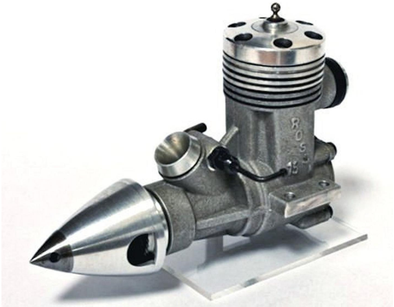
Rossi R15 – 0.7 BHP at 25,000 RPM from 2.5 cc on straight fuel, circa 1973.
