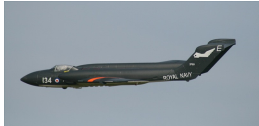
DH110 Sea Vixen. 1M Wingspan, weight 1.4kg, powered by 4S 900W Leopard fan
