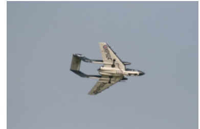
DH110 Sea Vixen. 1M Wingspan, weight 1.4kg, powered by 4S 900W Leopard fan
