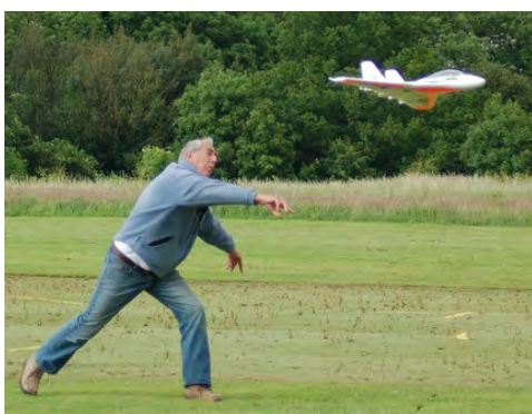
LEFT: David Whiteley puts a bit of gumption into hand launching the delta that set what must be an Olympic record by earning WLMAC the first noise complaint about an electric model. Measured on the club's sound meter, the pusher prop-powered screamer registered 84.5 decibels while airborne and an excruciating 94.5 decibels at a distance of seven metres on the ground. (Legal limit is 82 decibels.) David was just helping out at a specially-authorized flight at a club night at the field. The man on the sticks reckons he's had enough publicity about his sound machine, so we'll leave his name out of it this time..
