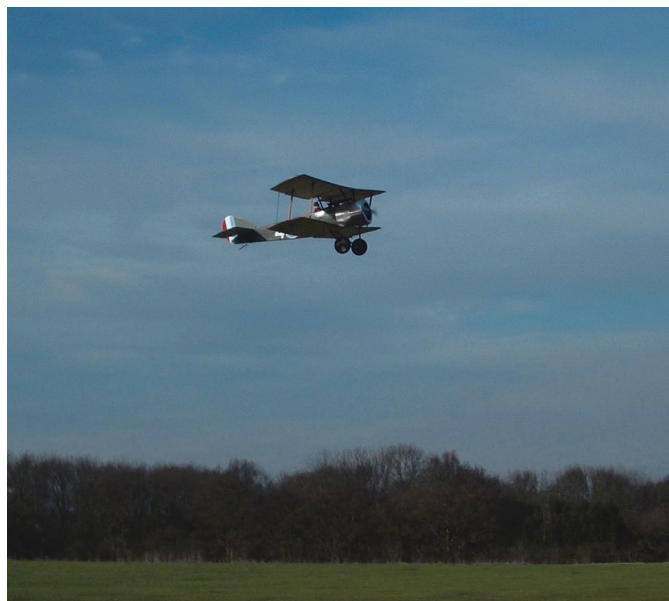
Brian Lee's quarter scale Sopwith Pup which he flies in a delightfully scale like manner. Fitted with a Laser 4 stroke twin, it has a subdued exhaust note that is convincingly realistic for an aircraft of this era.
