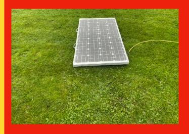
Now that the dull and gloomy days are here, the Solar panel is working hard to keep up with our demands. When we do erect the panel, if it's a gloomy day, place the panel flat on its back. If it's sunny, erect it and angle it to the sun. When it's dull, it will then collect energy from the whole sky rather than half the sky.
