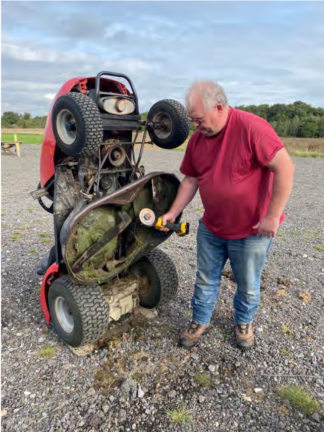
New parts being fitted to the ride on mower. Belts and pulleys and a quick sharpen of the cutting blades.
