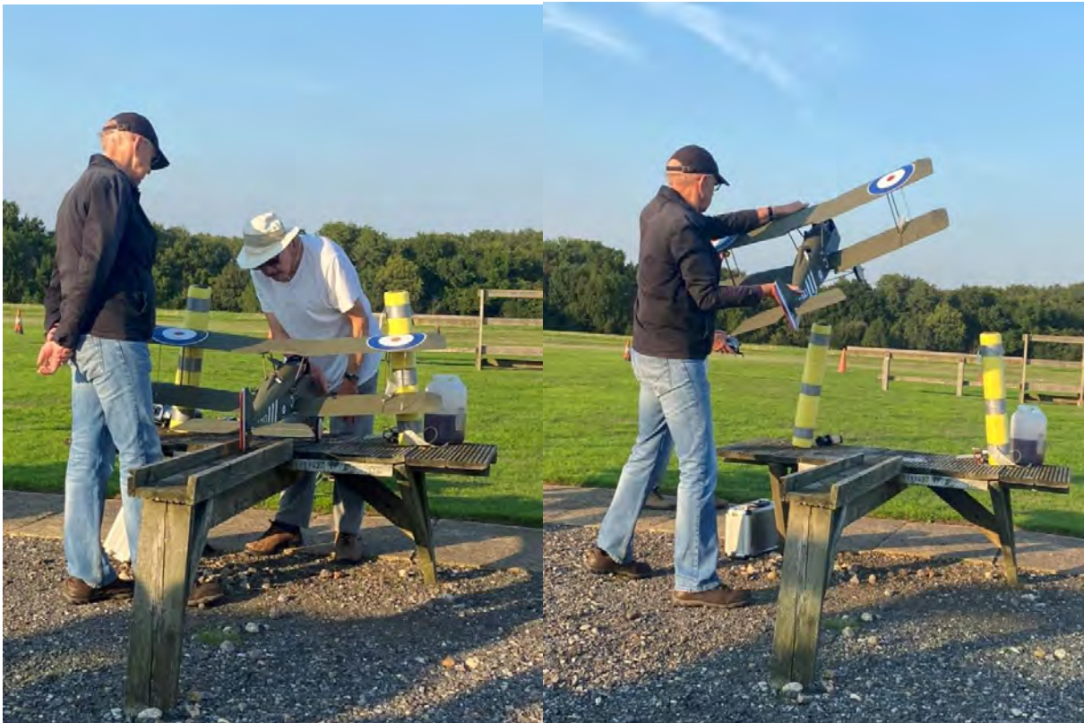
SE5A built from Flair Kit, 2 years in the build, 52" span, O.S.56Mk3 engine, by Frank Dalby-Smith. It's now had about 6 flights and so far, so good.
