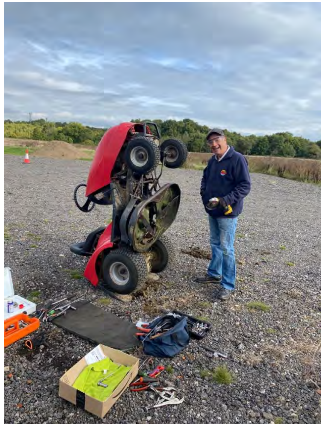
New parts being fitted to the ride on mower. Belts and pulleys and a quick sharpen of the cutting blades.
