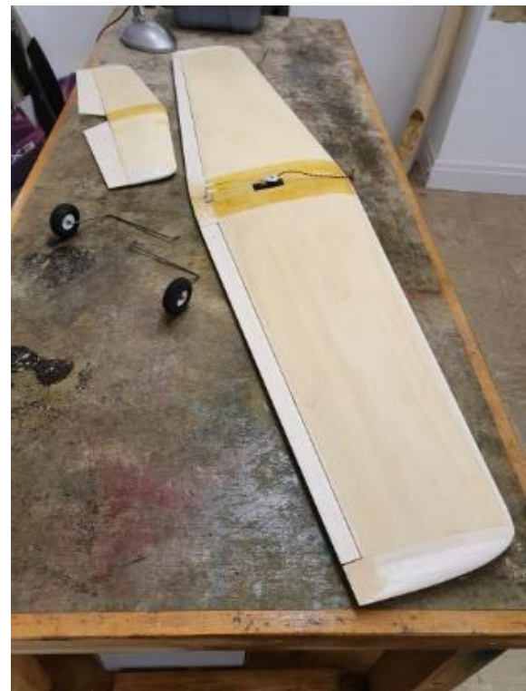
De-laminated tail and wings recovered with Obechi veneer with new tips etc, looking a bit less horrible now.
