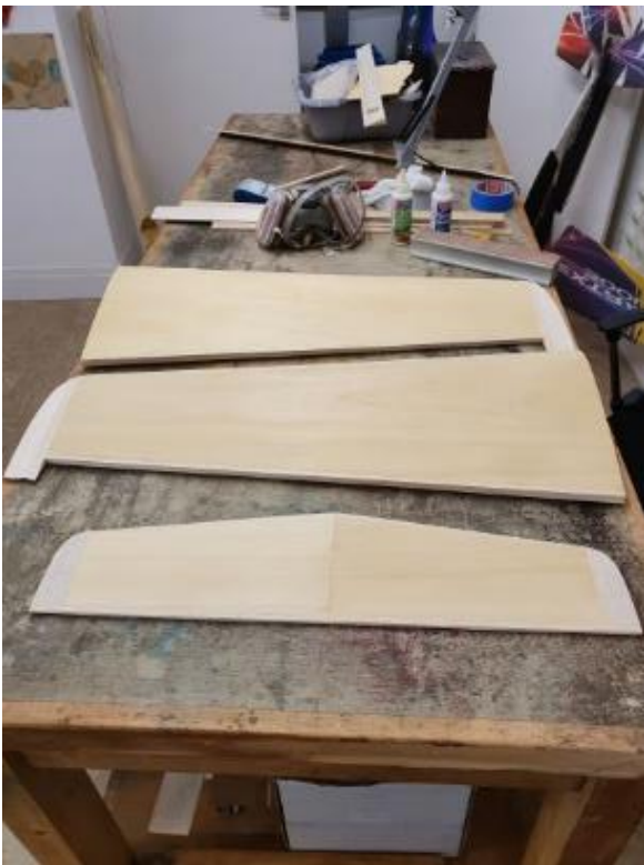
De-laminated tail and wings recovered with Obechi veneer with new tips etc, looking a bit less horrible now.
