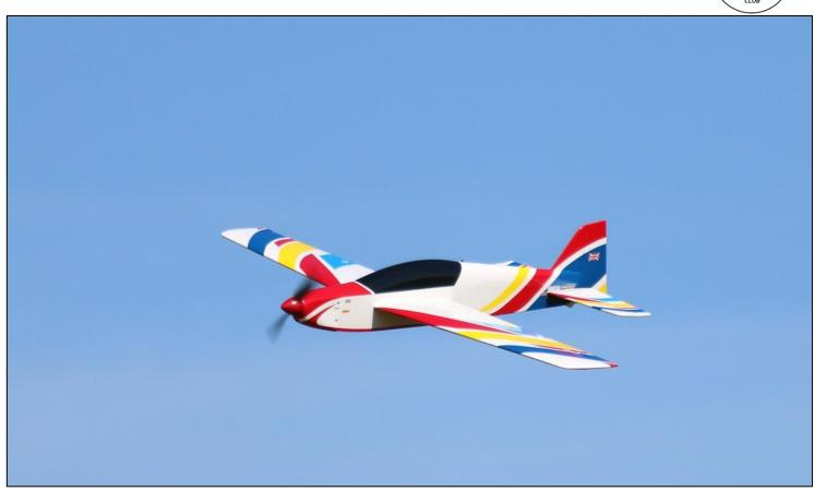
Colin Martin's Ripmax Easystreet 2 – wingspan is 44", it weighs 2.7 lbs and is powered by a 1200kv Quantum II motor with a 60amp ESC and 4 cell 2700 lipo. It flies fast but handles well at low speed, the timer is set for 8 mins but still has plenty in reserve. Good for any conditions, and is easy to hand launch.
