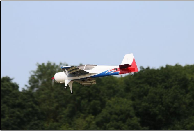
Michael Johnson's Sebart Sukhoi S29 30E – goes well on 4 cells (Sebart 30 series are fine in flat calm, but often struggle if there's any wind).
