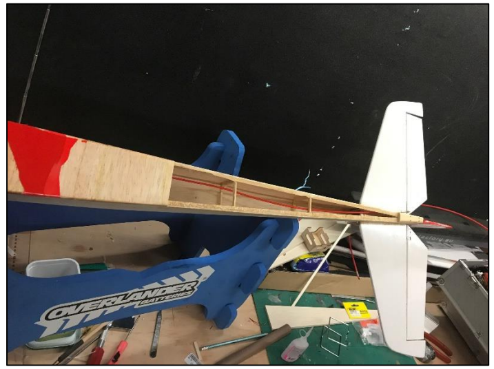
...and then take the bottom of the rear fuselage off to reveal a completely unsupported snake - this is never going to work because unlike (say) a bowden cable on a bicycle, the clearances are far too loose. Snakes are normally fine if you support them every 3-4 inches.
