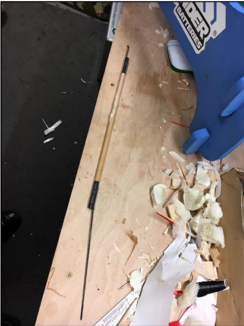
Graham went for the Rolls-Royce solution and installed a closed-loop system on the rudder, which sits nicely with the original elevator pushrod shown here.
