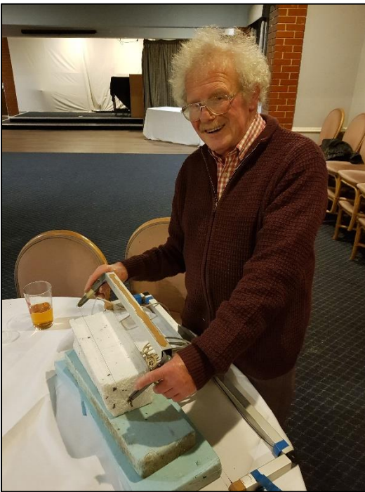
Dave Chinery using nichrome wire in tensioned bow running off a Lipo or Nicad (voltage to suit wire length / resistance / type of foam)
