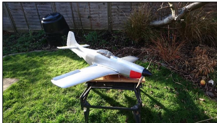
The P-51 covered and ready to go – not much scale detail, but in the air it's definitely a Mustang. Power is from a 6s5000 LiPo, the 4-max 360 kv motor turns 16" x 10" prop. Flight time is 6 minutes with plenty of battery left so 8 minutes of warbird-type flight should be achievable.
