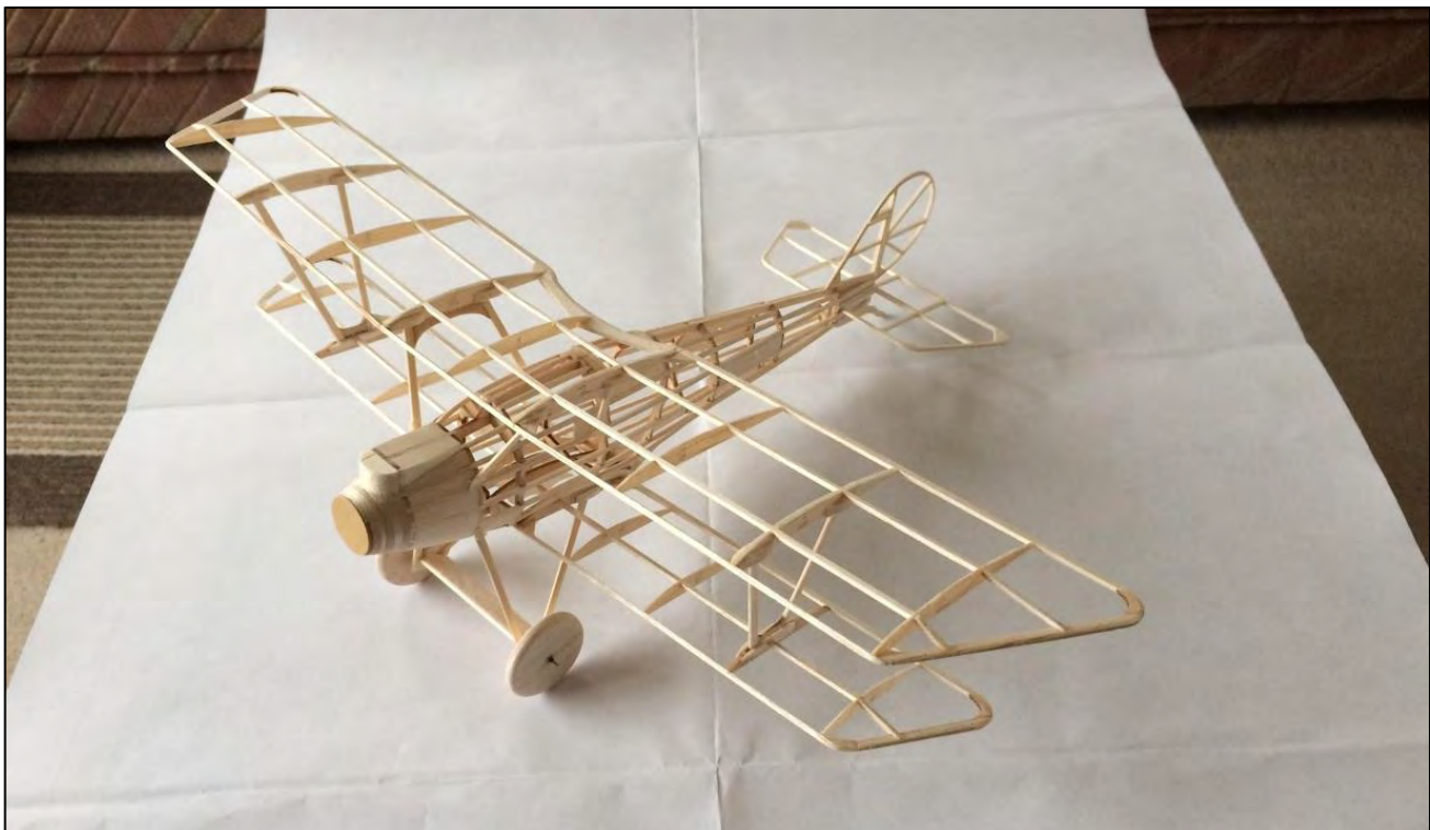
DPC Models Pfalz D.III. Model is 16" span and weighs about 11.3 grams in this bare-bones state.
