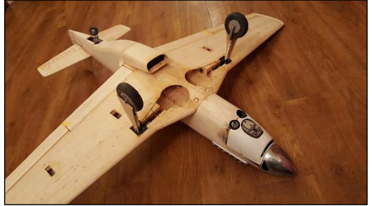
Underside showing retracts and flaps
