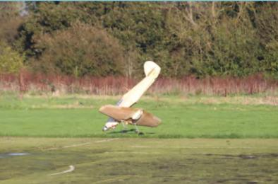
The sacrificial plastic wing bolt then did its job and broke apart allowing the wing to part company.
