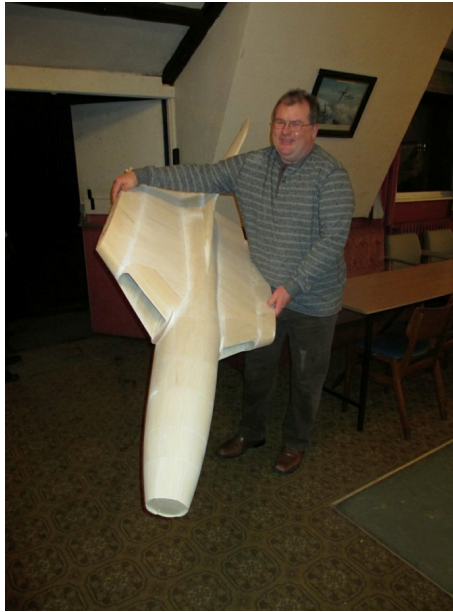
Tony is designing three different sized Vulcans. This is the largest, designed for one single turbine that exits down the middle. Chairman Mat wonders if it will fit in his van.....
