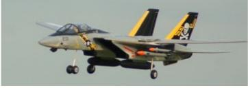
Festooned with dummy fuel tanks and missiles, this US Navy Tomcat is the latest addition to Harefield's stable of ducted fan foamies, cutting a colourful military dash on final approach to the strip. There are two electric ducted fans in the fuselage and the swing wings – seen here extended for the landing — are fully functional. Undercarriage is retractable. Owned and assembled by Stewart Wilkinson, the Tomcat performs to the skilled hand of John Smith.
