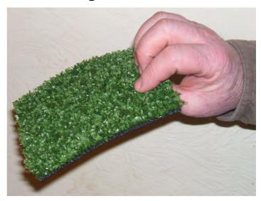
Above: This is Astro Turf— a layer of man made fibres, 12 mm thick, mounted on an extremely tough backing. It comes in rolls and is professionally laid on a bed of sand on levelled ground. Rainwater drains straight through it. Harefield's natural grass would butt up to its edges. Come to the AGM to hear all about it, express your views and cast your vote for or against its use.
