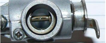
**LIVE AND LEARN DEPARTMENT** Hours of fiddling with the slow running needle on the ASP120 four stroke installed in Tony Taylor's newly acquired Stearman biplane failed to persuade it to tick over when it was throttled back. It just stopped. But a very close look indeed inside the carburettor found the trouble. A giant split in the spray bar. Cause of the problem identified!
