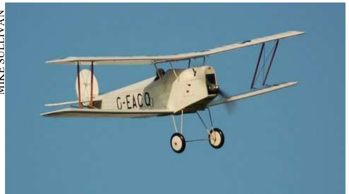
Tony Taylor's natty little "Avro Baby" which is, believe it or not, rudder and elevator with no ailerons photographed at Harefield in mid October.
