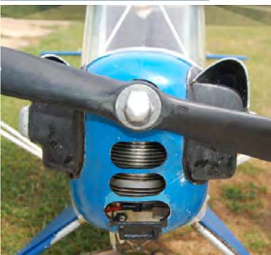
LEFT. It is rarely that weather-related engine overheating is a problem for us but during the mid-year heat wave the Laser 150 in Leon Taylor's much-flown clip wing Cub ground to a halt in the air. The PTFE plugs that cap the ends of the piston gudgeon pin had melted and spread themselves between piston and cylinder wall. It could have been worse. Leon soon had his Cub back in the air, with more holes in the cowling to keep that big cylinder cool in case the heat wave should return.
