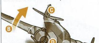
**C.** The low airspeed means the rudder is not effective enough to counter the yaw
