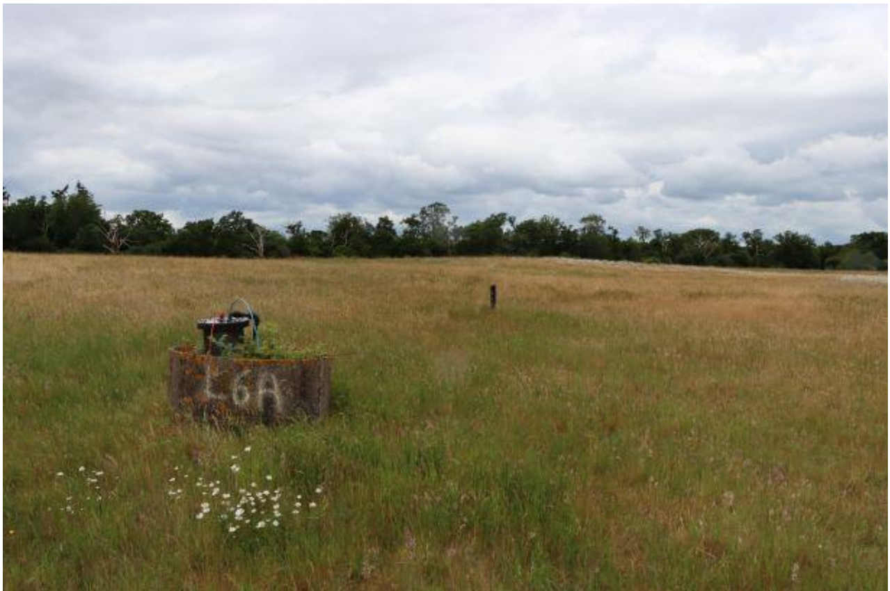
Suez have offered to lower some gas monitoring points to ground level, placing manhole covers over them.
