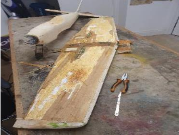
Stripped down to basics, even the foam was damaged
