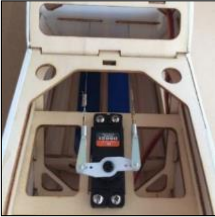
Rudder servo in place. The supplied closed-loop wire was heavy-duty (circa 0.7 mm) which isn't necessary on a model of this size, so it was swapped for some closed-loop wire that I had lying around. Mole grips were useful for crimping the wire.
