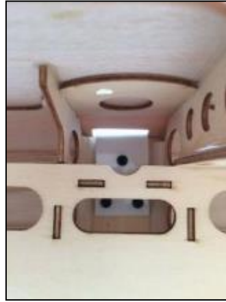
The Angel 50 undercarriage is reasonably robust (extremely so for an ARTF) and the legs are fixed in place with three M3 bolts. However, the left and right legs look very similar and it's easy to get them the wrong way round.
