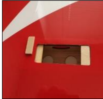
I used some older but perfectly serviceable standard-size digital servos that had previously been in a Kyosho Osmose 50, but the wing servo mounts needed a 2 mm ply shim to lift them up a bit.
