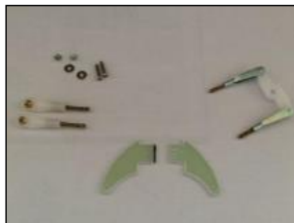
The closed-loop connector set for the rudder - one of the rudder horns did need trimming as shown by the black line, and I elected to use some standard M2 clevises on the rudder servo because the supplied nylon ball-link clevises were difficult to adjust.
