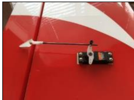
Aileron servo installed, all pretty straightforward stuff.
