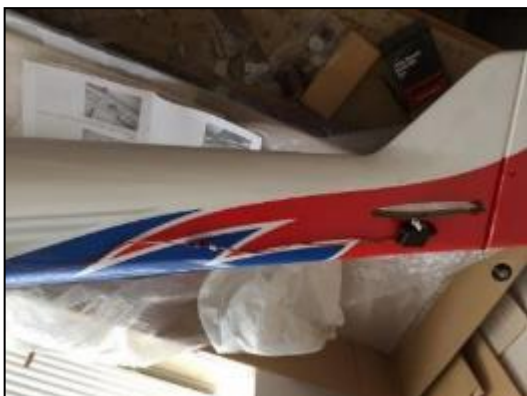
Checking the elevator servo lead length, this one needs a proper keeper on the connector because if it comes off, it's curtains.
