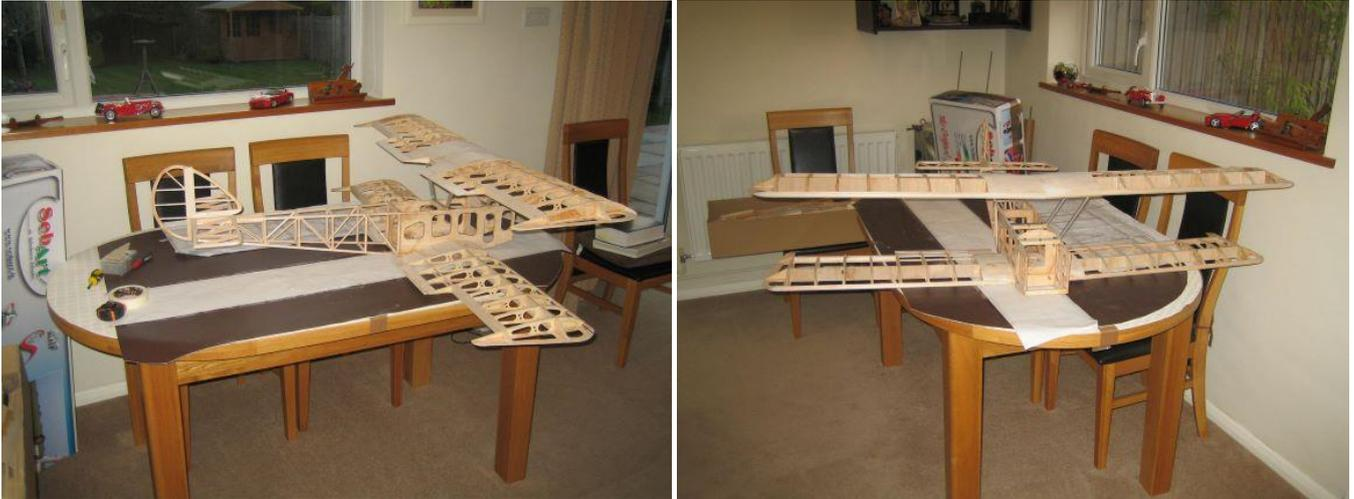
Just a quick couple of pic's to show progress & first fit of wings. They need a bit of alignment but should work out ok.
