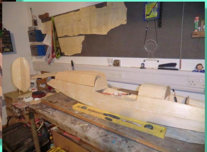
Here is Roy Lannings B24 Liberator which he's building from a Jack Stafford Kit purchased in 1979. The model has a wing span 90 inches with the original power was for 4 x 25 engines but is now being converted to electric.
