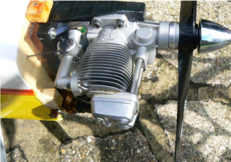
Restored to the Acrowat, same problem. But this time some movement of the engine in the airframe was spotted and the problem diagnosed. As the engine moved forward under power the throttle linkage moved the lever arm back causing a reduction of thrust and allowed the engine to resume its normal position. This caused the throttle lever to move once again causing revs to increase in the process. And so this "hunting" cycle continued.
