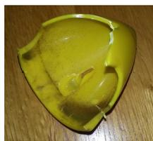
broken spinner clear to see when the blood had been washed away. What precautions might have been taken? Well if you're freeing up a dry and stiff engine—especially if it is of substantial size, lubricate it lightly with just a drop or two of light oil (not fuel) in the right places—down the plug hole, into the carburettor barrel and turn it by
